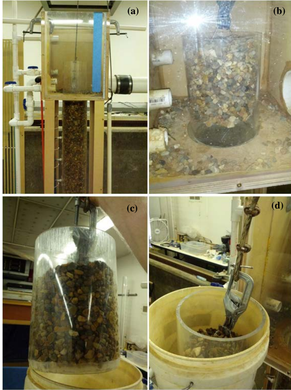
Figure 3.9. Method of retrieval: (a) plexiglass insert inside the headbox with hook, cable, and pulley to retrieve wire baskets; (b) pulling gravel into clear acrylic section. This photograph shows with “clean” pea gravel (without fine sediment deposited on it); (c) pulling with upward force, the natural heave of gravel locks it inside the clear acrylic section and allows it to be transferred into a collection bucket; (d) placing retrieved layer into bucket. When the clear acrylic section is lifted off, the gravel falls out into the collection bucket.
