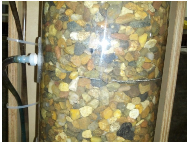
Figure 3.8. One of the wire baskets buried in a layer of pea gravel
