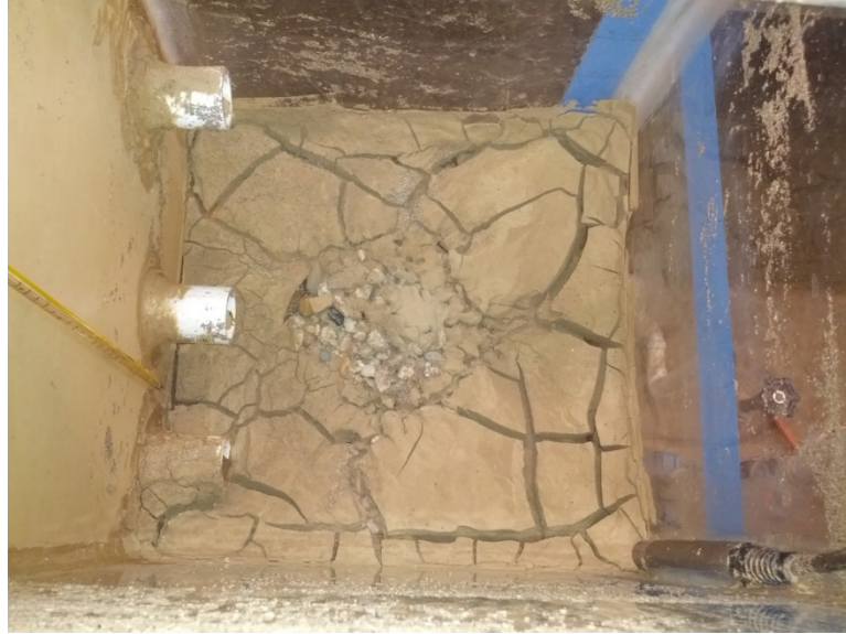
Figure 4.22. Dried sediment at the surface of the permeameter.
