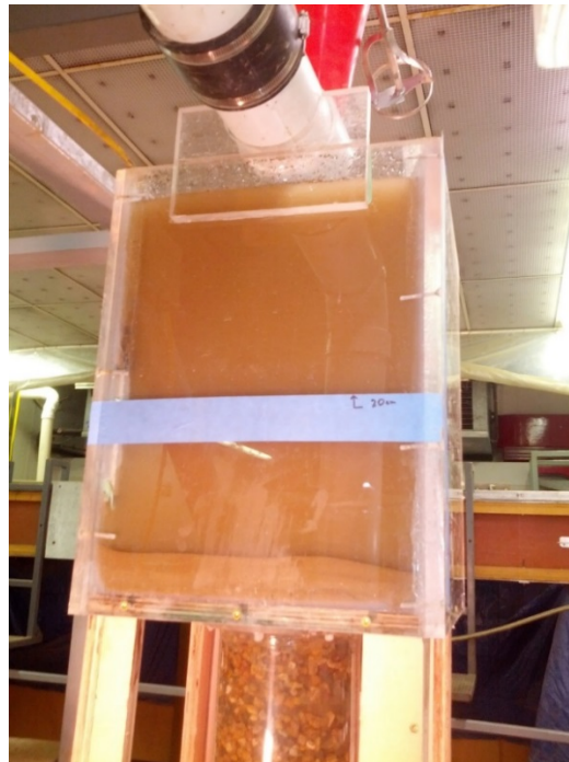
Figure 4.20. Sediment deposited in the head box during an experiment.
