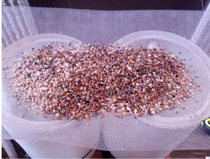
Figure 3.3. Washing gravel through stainless steel mesh (No. 10 (4.75 mm) sieve size)
